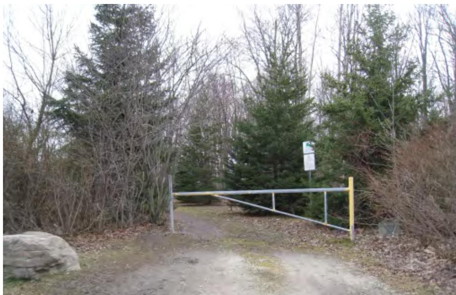
*An Example of a Swing Gate, Aurora, ON (note that this gate does not provide a permanent opening to allow trail users to flow through freely.)*
