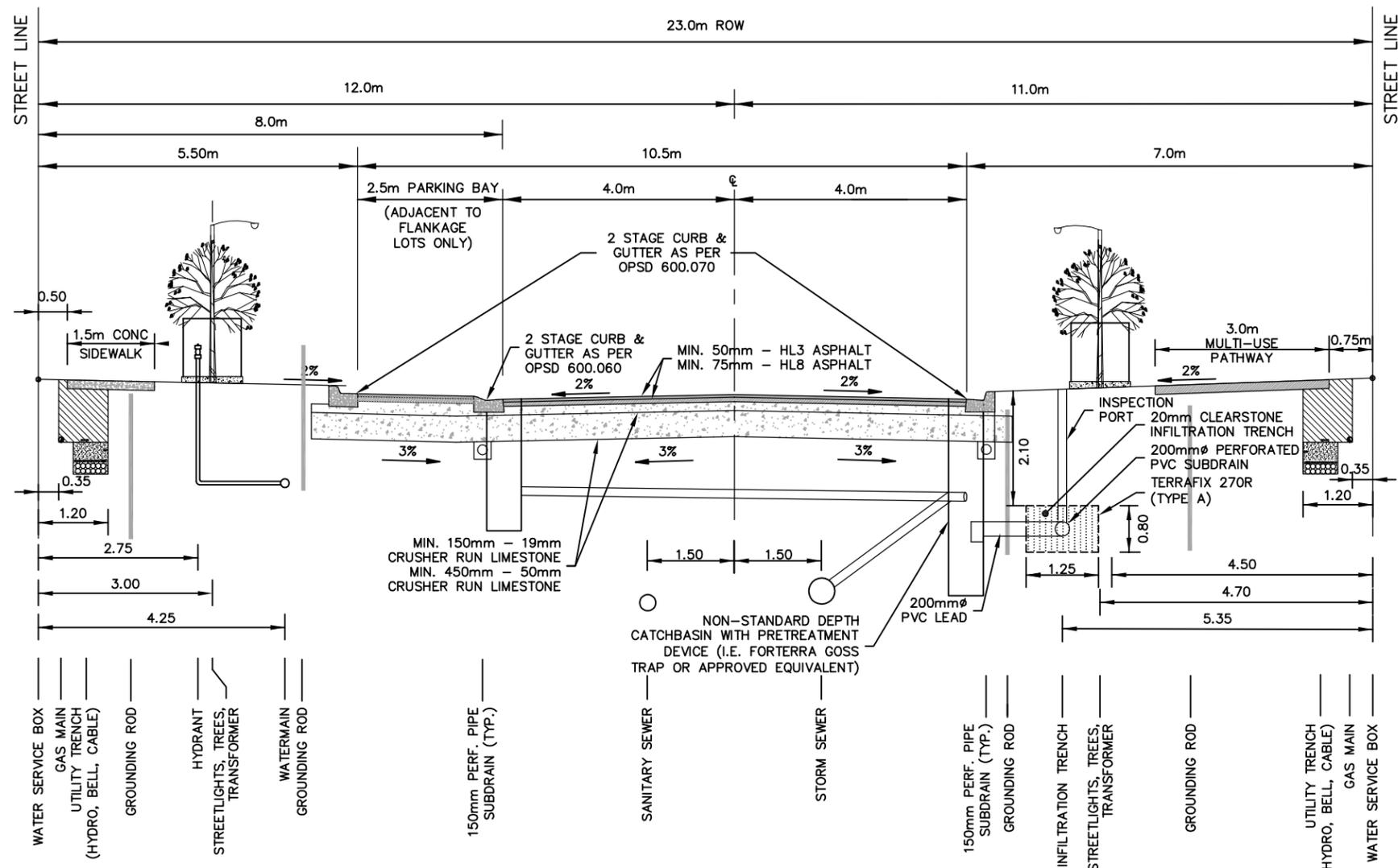
\*NOTE: LAYOUT IS SCHEMATIC ONLY, DETAILS TO BE PROVIDED AT DETAILED DESIGN STAGE.
