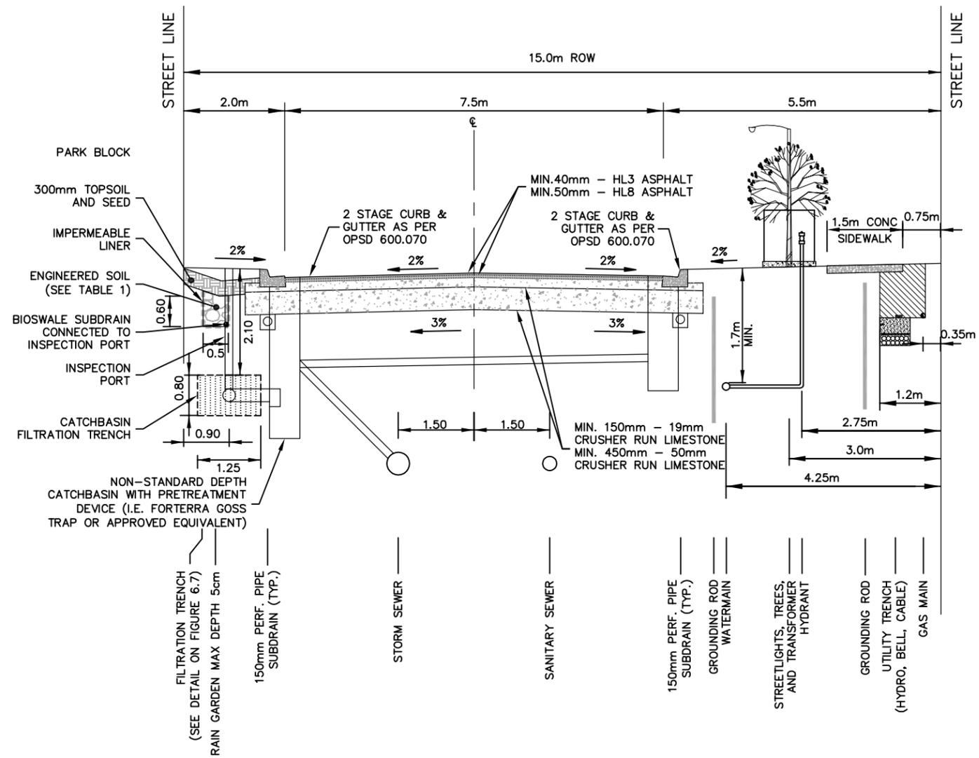
\*NOTE: LAYOUT IS SCHEMATIC ONLY, DETAILS TO BE PROVIDED AT DETAILED DESIGN STAGE.
