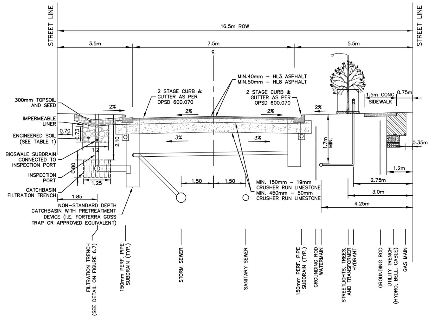
\*NOTE: LAYOUT IS SCHEMATIC ONLY, DETAILS TO BE PROVIDED AT DETAILED DESIGN STAGE.
